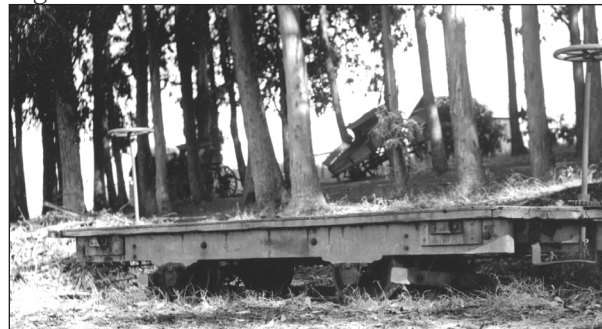
Narrow-gauge railcars used at Pt. Isabel to carry powder
