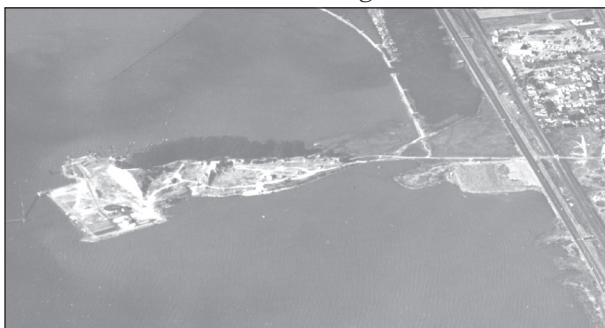
Pt. Isabel after the west end of the hills had been cut off for the Stege Sanitary sewer plant. The cut is clearly visible
